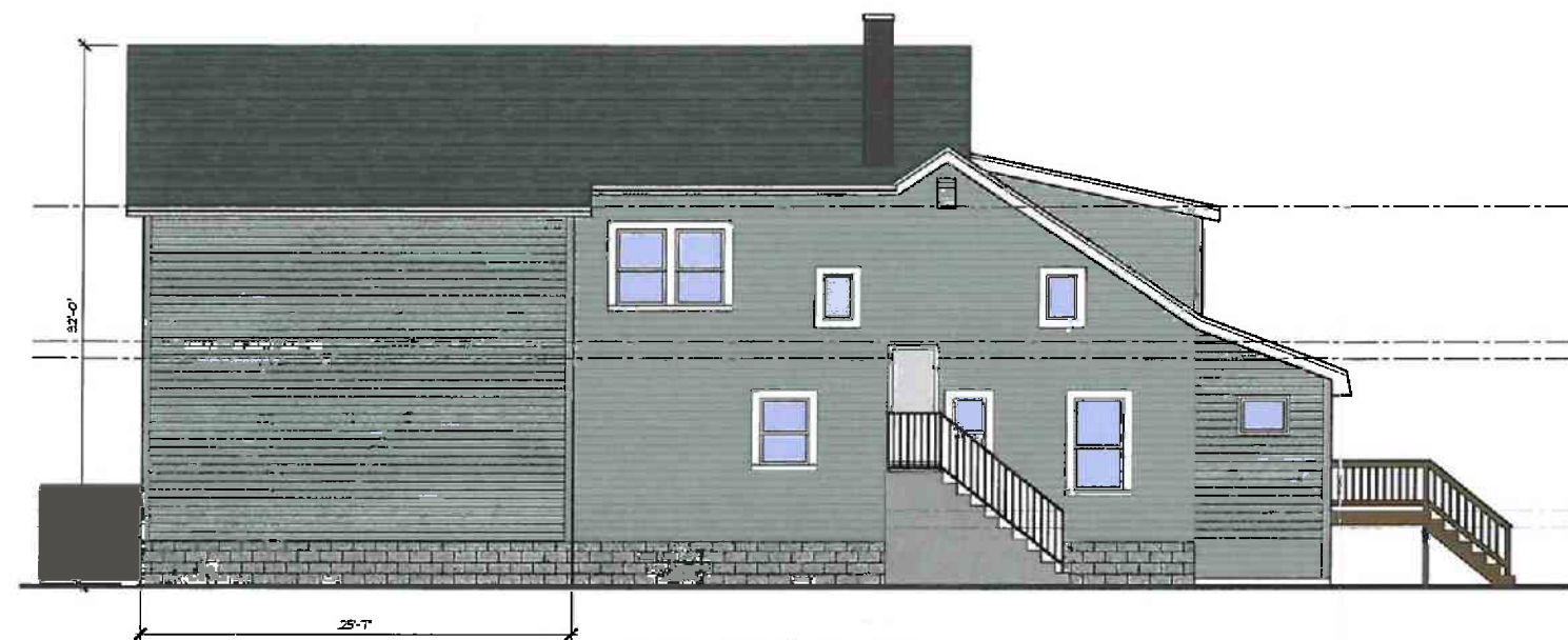
4 NORTH ELEVATION SCALE 3/8" = 1'-0" 0 2 4 6'
